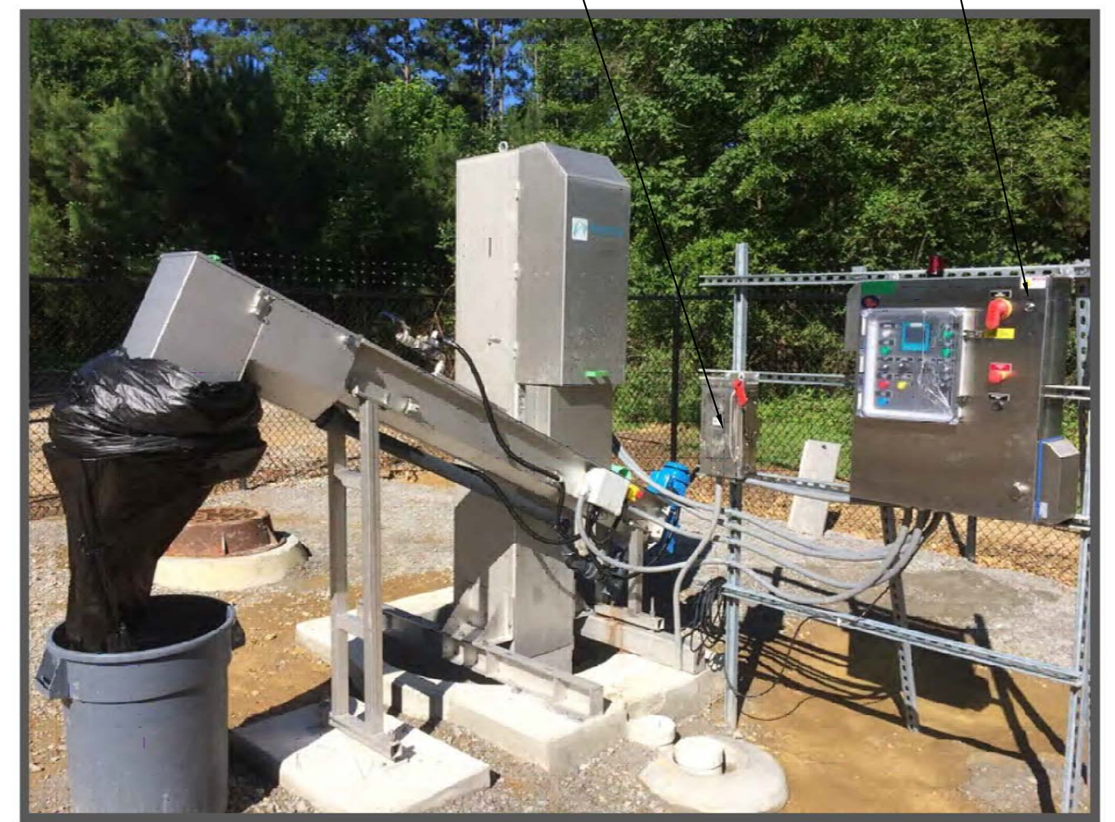
TYPICAL SCREENING/WASHER UNIT ASSEMBLY (FOR REFERENCE ONLY)
